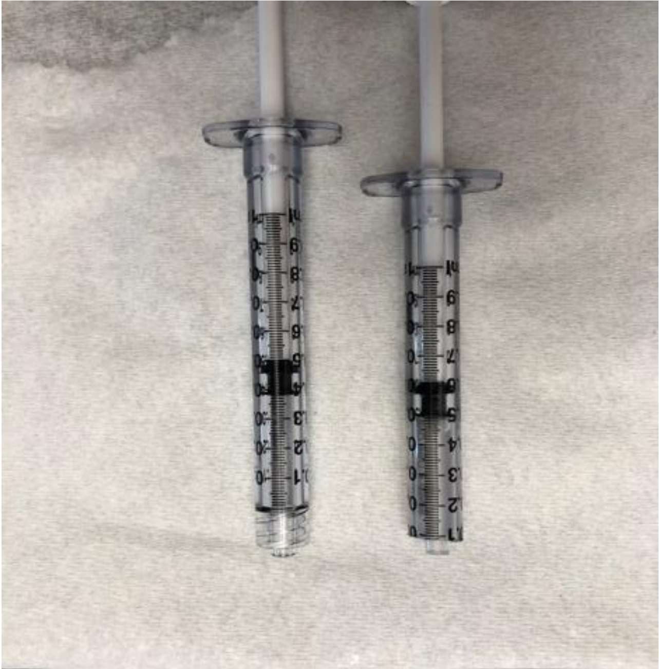
Figure 3: 1mL syringes used to make agarose plugs. The syringe on the left is unmodified. The syringe on the right had the end cut off and was used as a mold to form agarose plugs (a piece of the plug is sticking out of the open end).
